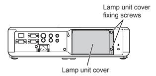
3) Use a Phillips-head screwdriver to loosen the 3 lamp unit fixing screws. Pull the used lamp unit gently from the projector.
