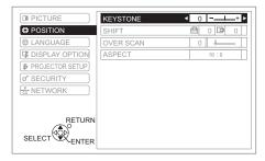
Press ▲ ▼ buttons to scroll to the required sub-menu item and press ◀► buttons or the ENTER button to adjust.
