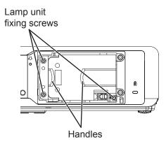
4) Press in the lamp unit until it clicks and make sure the unit is installed securely. Tighten the 3 lamp unit fixing screws securely with a Phillips-head screwdriver. When inserting, in particular press the portion of (A) securely.
